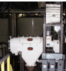
CENTRI-SIFTER screener simultaneously mixes a flow aid with finely ground rubber, breaks up soft agglomerates and removes fiber and steel debris from on-size material.
