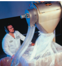
Large toll processor screens plastics, additives, foods and pharmaceutical products using mobile CENTRI-SIFTER screeners configured on caster-mounted stands.
