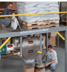
Producer of aquaculture feed, high in lipids, screens down to 300 microns (0.3 mm) 60-times faster than with vibratory screener while eliminating screen blinding.
