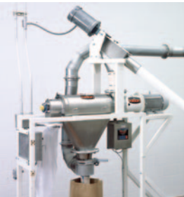
Producer of 200 dairy blends having bulk densities of 25 to 60 lb/cu ft (400 to 960 kg/cu m) screens directly into sacks by weight at rates to 25 lb/min. (11.3 kg/min.)
