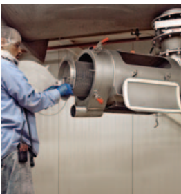
Blender discharges into low profile, QUICK-CLEAN, CENTRI-SIFTER screener that removes oversize particles and discharges on-size material into mobile storage vessels.
