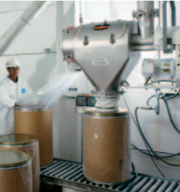
Toll processor scalps cryogenically-ground engineering resins at -50° to -275°F (-46° to -170°C). QUICK-CLEAN design allows changing of screens before ice can form.
