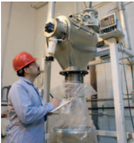
CENTRI-SIFTER screener removes oversize particles from on-size powders at temps to 450°F (233°C) and rates to 1000 lb/h (453 kg/h) while reducing agglomerates.
