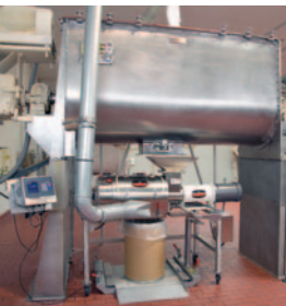
Compact CENTRI-SIFTER screener fits a restricted space between a blender and fiber drums being filled with 100 lbs (45 kg) of screened food ingredients.
