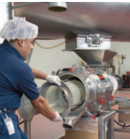
Flavor powder producer switched from a vibratory screener to a QUICK-CLEAN CENTRI-SIFTER screener, boosting output 150 percent while cutting wash down time.
